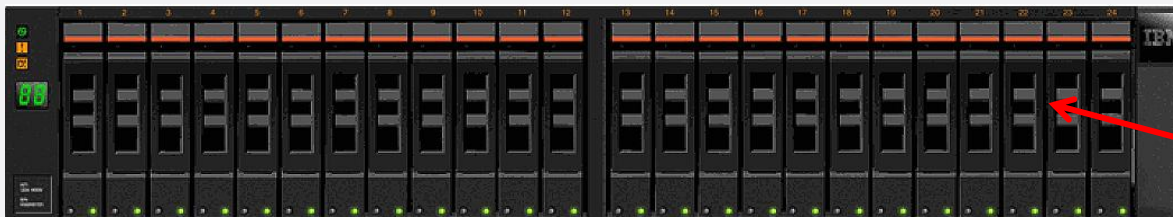
Storwize v7000 expansion enclosure 2076-224
